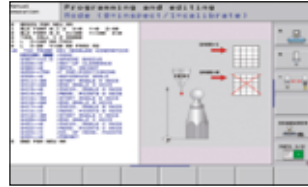
KinematicOpt & kinematicCon option Touch probe cycle for automatic measurement
